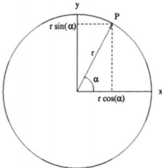
Figure 10: Relationship between polar and rectangular coordinate systems.
