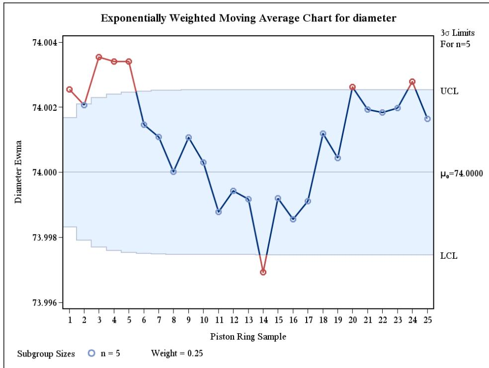
**EWMA Chart for Piston-Ring Diameters with Resets
