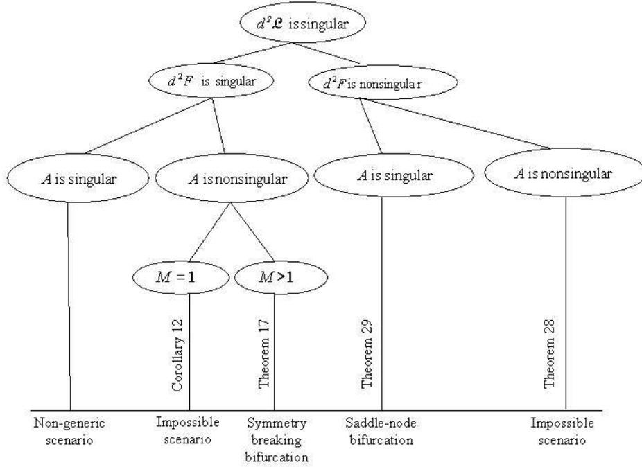
Figure 7: A hierarchical diagram showing how the singular points of  $d^2\mathcal{L}$  and  $d^2F$  affect the bifurcation structure of equilibria of (20).
