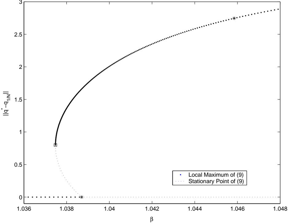
Figure 6: The subcritical bifurcation from the solution branch  $(q_{\frac{1}{4}}, \beta)$  with symmetry  $S_4$  to a branch with symmetry  $S_3$  at  $\beta^* = 1.0387$ . This was predicted by the fact that  $\zeta(q_{\frac{1}{4}}, 1.0387, 1, 3) < 0$ . The bifurcation diagram is shown with respect to  $\|q^* - q_{\frac{1}{N}}\|$ . It is at the saddle node that this branch changes from being composed of stationary points to local solutions of the problem (9)
